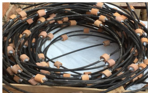
Fig. 2: Hoses of innovative follicular (porous) drippers before installing in experiment site.
